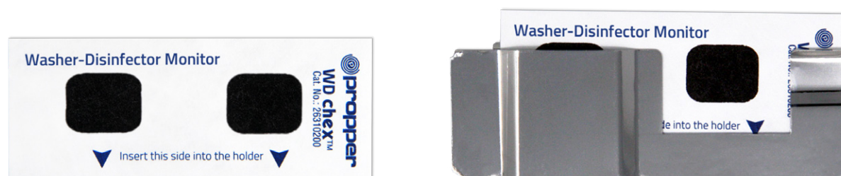
Figure 1. Proper WD chex™ washer-disinfector. Left image shows loose monitor. Right image shows monitor in designated holder.
